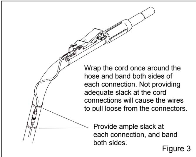
**2.2.5** Band the cord to the blast hose every 4 to 6 feet. Also, band the cord on both sides of electrical connection.
