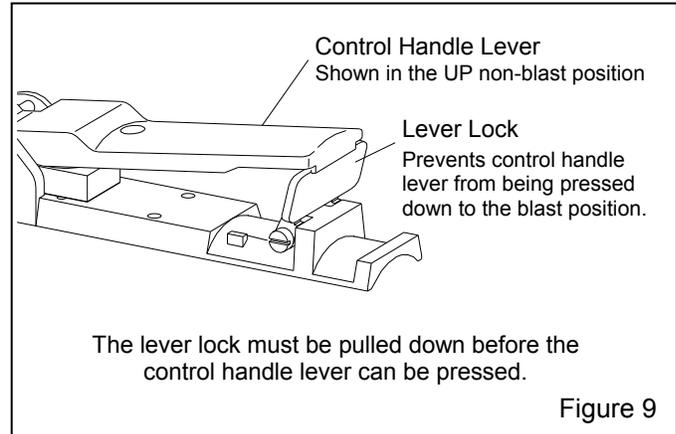
**3.2.11** Make sure the handle lever does not engage the switch unless the safety lever lock is intentionally pulled down.
