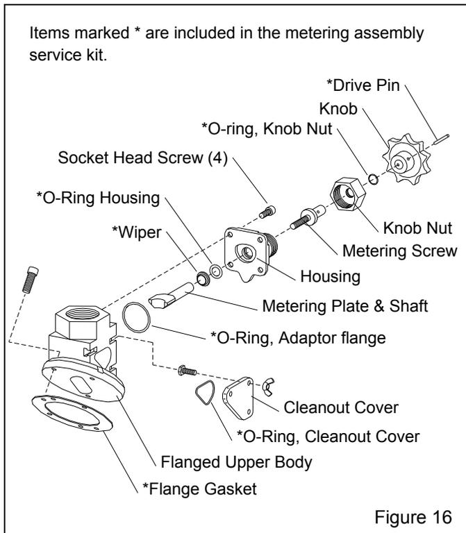
**6.6.4** The flanged upper body and actuator do not need to be removed from the blast machine to service the metering assembly. Thoroughly inspect both items for wear, and replace if worn.
