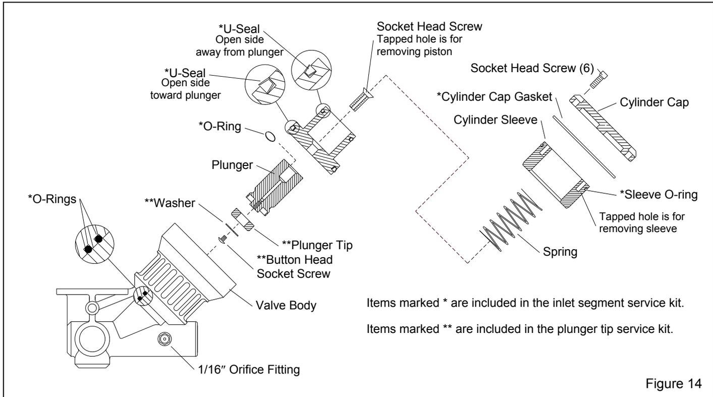
**6.3.7** If the plunger and piston were separated as noted in paragraph 6.3.4, apply removable thread sealant to the socket head screw, and reassemble the parts using a new o-ring supplied with the service kit.
