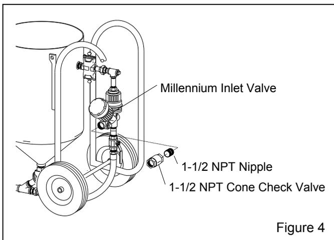
**2.3.1** Where multiple blast machines are operating from a single air source, install a check valve at the air supply on each machine. The illustration in Figure 4 shows where to install a cone check valve on the blast machine.
