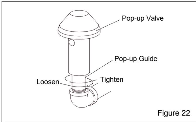
**6.10.5** Slide the new pop-up valve over the guide, and then screw the valve guide (with the pop-up valve on it) into position inside the machine. Tighten the guide, it should be wrench-snug, but not wrench-tight. Over-tightening the guide will make it difficult to remove the next time the pop-up valve needs replacement.
