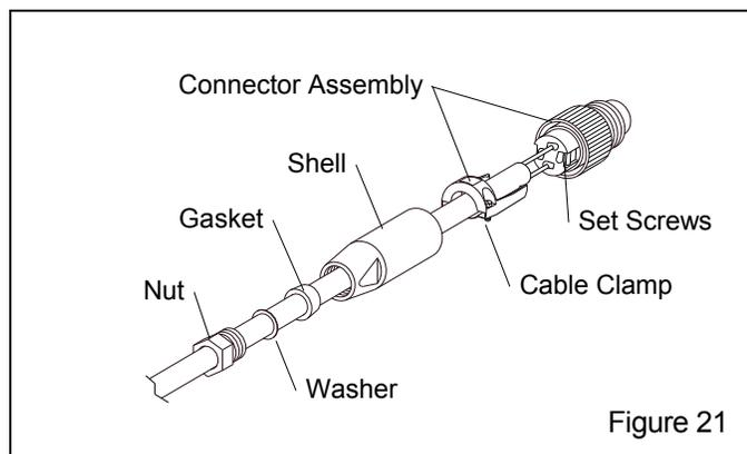
**6.8.4.4** Remove the shell from the insert assembly.
